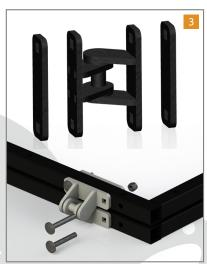
Where there will be a drop bolt mounted, it is necessary to insert the head of the bolt on the inside of the leaf. In all other places, fit the bolts such that the head of the bolt is on the exposed face of the gate. This results in the nut being protected from any tampering as it is shielded by the mesh/hoarding panels.
